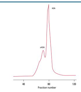
Resin: **TOYOPEARL HW-50S** 22 mm ID  $\times$  83 cm Column size: Mobile phase: 10 mmol/L HCI Flow rate: 1.6 cm/hr (0.1 mL/min)
