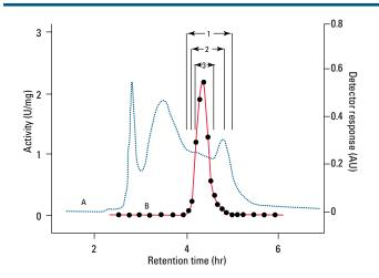
Resin: TOYOPEARL HW-55F Column size:  $25 \text{ mm ID} \times 55 \text{ cm} \times 2$  Mobile phase: 0.2 mol/L phosphate, pH 6.7 Flow rate: 12 cm/hr (1.0 mL/min) Detection: A. UV @ 280 nm
